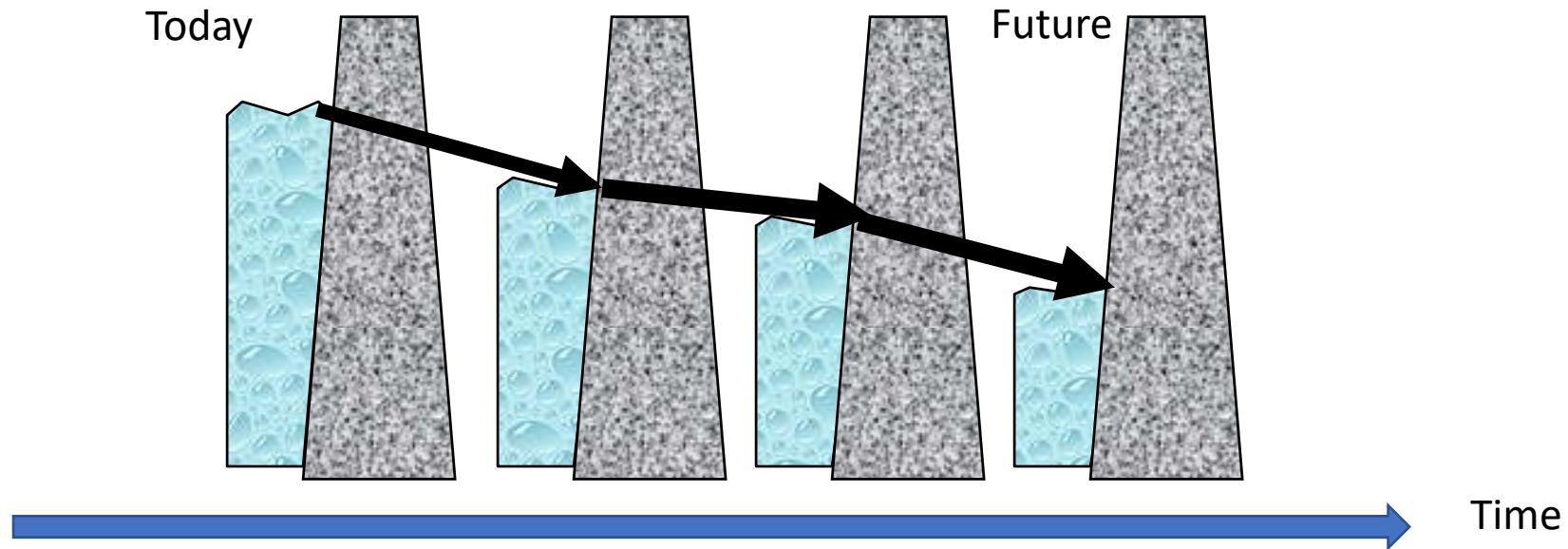
Future water storage depends on present storage, future water inflow and the decision about how much thermoelectricity could be substituted by hydroelectricity
