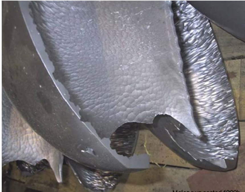
Fig 1: Eroded Buckets of Pelton Runner
