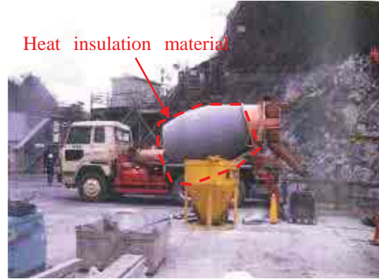
Photo 3: Mixer vehicle with heat insulation material attached
