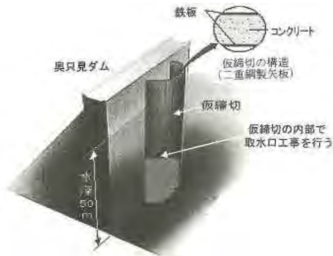
Fig.11: Outline of the makeshift cofferdam
