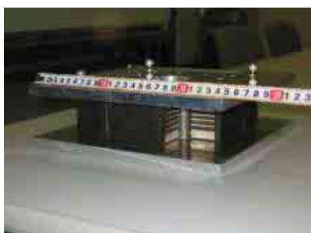
Fig. 6: Model of Aseismic rubber bearing (LRB)
