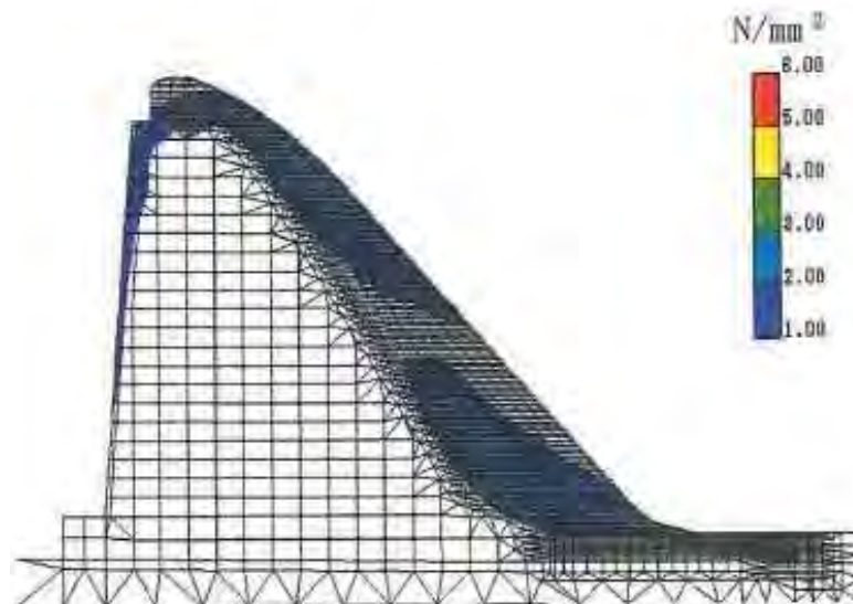
Fig. 3: Thermal stress analysis results
