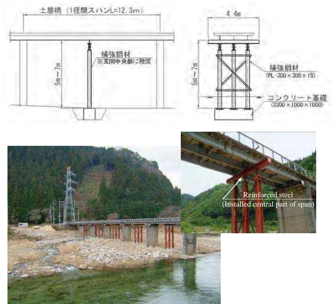
Fig. 5 Conceptual diagram of the Doi bridge reinforcement and the construction works status
