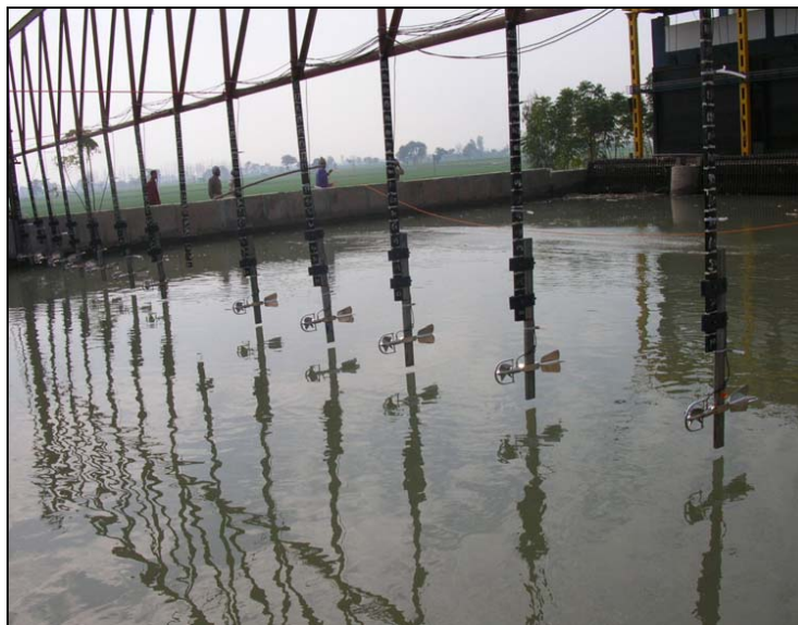
Fig. 17 (b) : Frame raised to pull PCMs out of water
