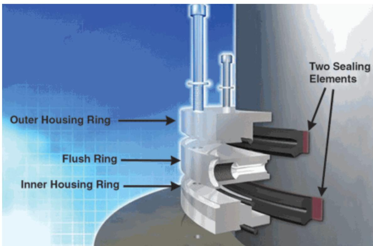
This split-type HydroSele cartridge seal was installed on the turbine shaft at the 5-MW Foyers Falls plant to reduce water leakage. The seal features two elastomer-based rotary sealing elements working back-to-back with flush water introduced between them instead of a typical mechanical face sealing arrangement.
